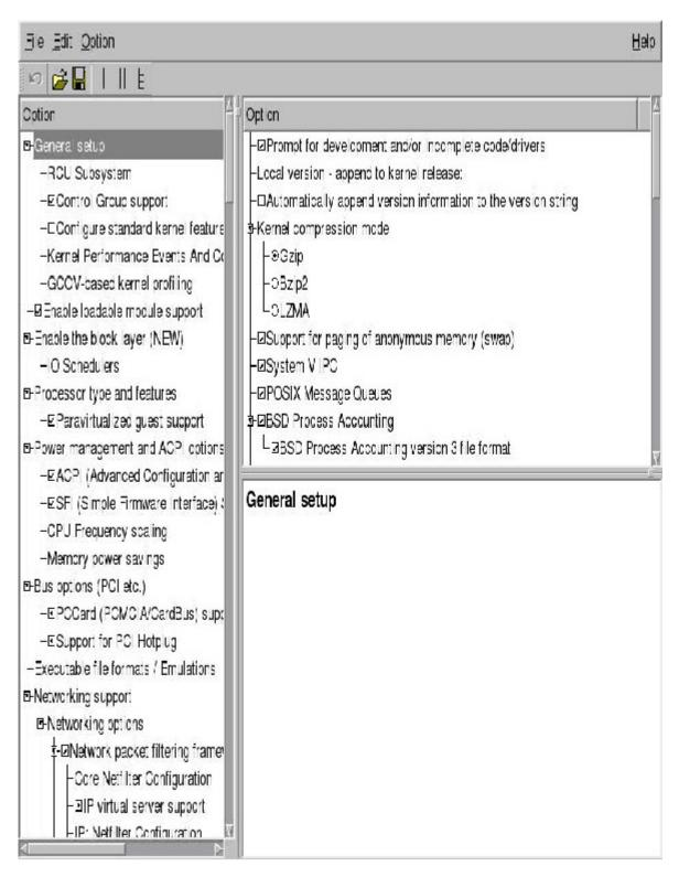
As said, the command make gconfig does exactly the same, but uses GTK instead of QT:
