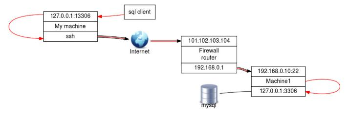
First open the tunnel by running ssh with the \"-L\" option:
