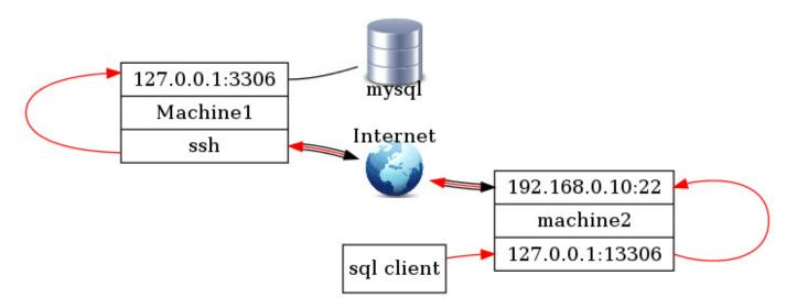
The tunnel will stay open as long as the SSH session is running or as long as there is a tunneled session going through it. This means there are two ways of working with SSH tunneling:
