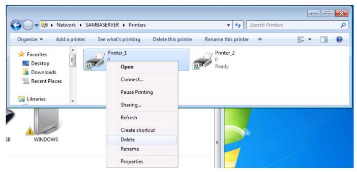
Right click enables connecting to the printer and adding it as a Generic text based printer.
