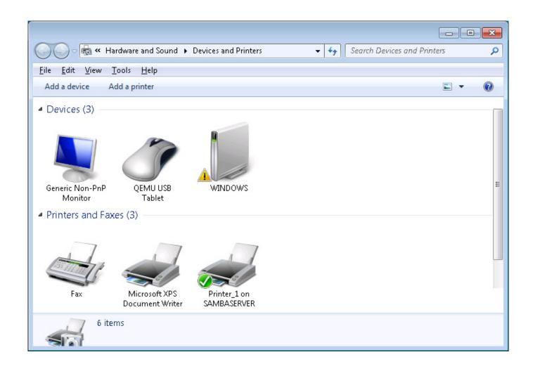
Right click Printer\_1 and print test page. Checking the spool file of the printer on "sambaserver":
